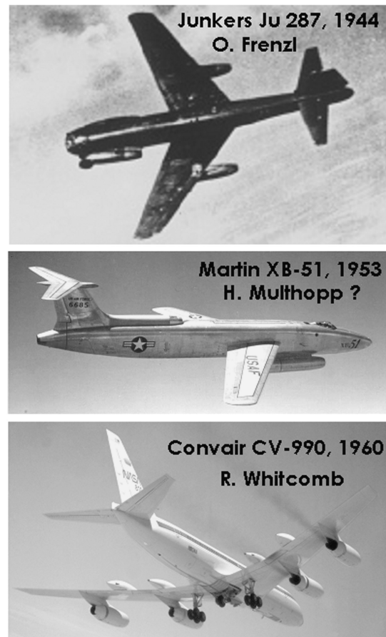
Fig. 40 Beginnings of transonic area ruling.
